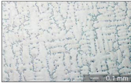
All ReCap™ Femoral Resurfacing components possess a high carbon, high carbide (> 20% carbide content) microstructure with “blocky” carbides resulting from a proprietary “as cast” argon shroud rollover processed raw material.
